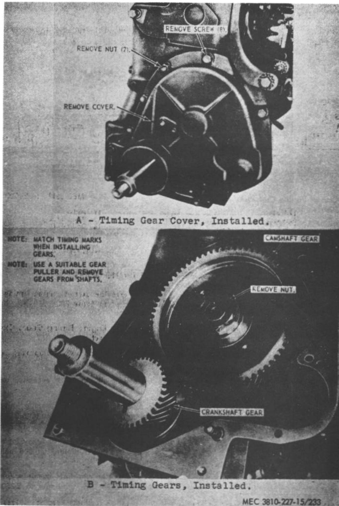
Figure 233. Carrier engine timing gears, removal and installation.
